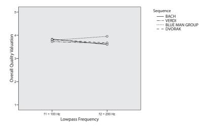
**Fig. 6.** Diagram showing the significant interaction between low pass frequency and sequence. The lower low pass frequency ( $f1 = 100 \, \text{Hz}$ ) is judged better in all cases except for the sequence Blue Man Group (BMG).
